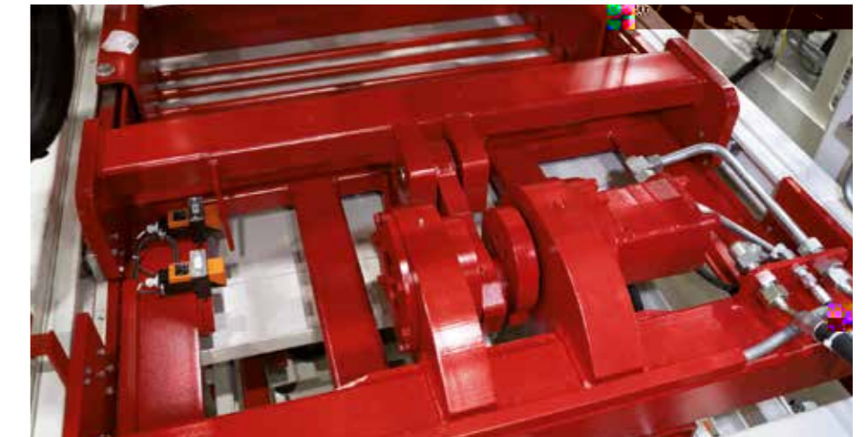
Hydraulically driven filler grid, for optimized filling of the mold and
