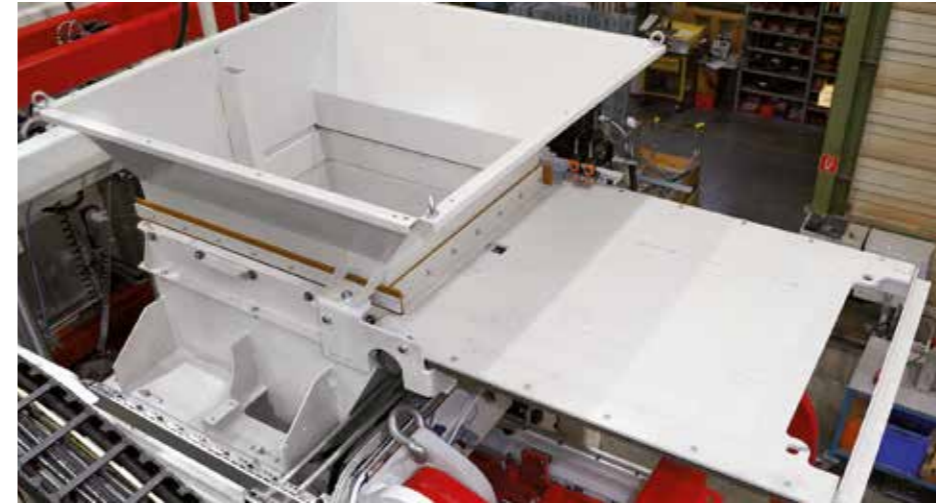
Colormix device with draw plate
