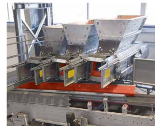
Color-Mix shuttle belt system
